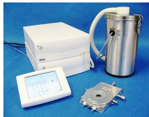
Geology System including LNP95 cooling system
