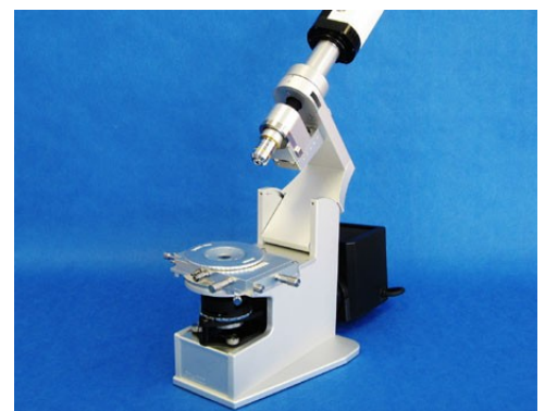
Linkam Imaging Station. Optics are tilted back to allow easy access to sample
