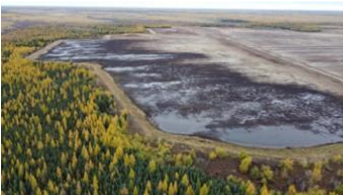
The Elma West peatland restoration site, mid-restoration, October 2023. The slope between the natural peatland (forest, left side) and the restoration area (brown, middle/right side) is clearly visible. Restoration will continue in fall 2023 and spring 2024.
